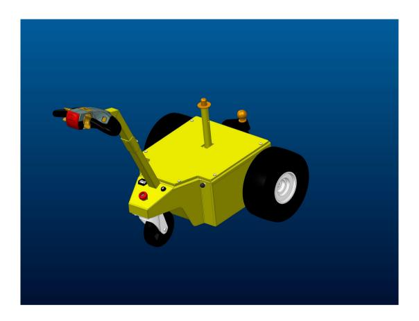
Tighten all wheel bolts to 120nm after the first 2 hours of driving.
