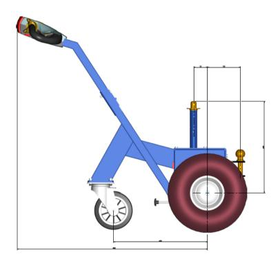
Tighten all wheel bolts to 120nm after the first 2 hours of driving.
