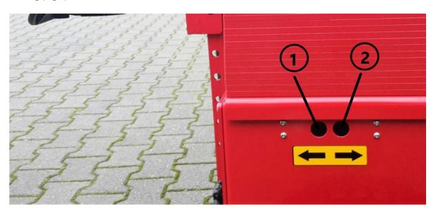
At the front left there are 2 buttons for moving slowly forwards (Fig 3, 1) and backwards (Fig 3, 2). Press the button 1 time to unlock, pressing the button the second time you can drive a couple of inches forward or backward. The maximum speed can be set using the potentiometers (Fig 2, 7 and 8) on the tiller head. The maximum distance you can travel in this way is approx. 1 metre.
