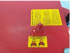
This model has 2 counterweight layers of approx. 600 kg each. You can lift these from the machine with 4 lifting eyes supplied. Screw these lifting eyes into the holes provided. (see photo). This way you can only lift the weight package and **not** the entire machine.
