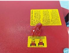
This model has 2 counterweight layers of approx. 600 kg each. You can lift these from the machine with 4 lifting eyes supplied. Screw these lifting eyes into the holes provided. (see photo). This way you can only lift the weight package and **not** the entire machine.
